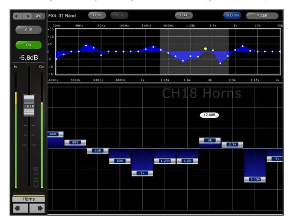
The current channel's Name, Color, Fader, Level Meters, [ON] and [CUE] buttons are shown in the left column. At the bottom-left, there are "previous" and "next" arrow buttons for navigating to different channels. Pressing these buttons will only access other channels that have GEQs assigned to them.
